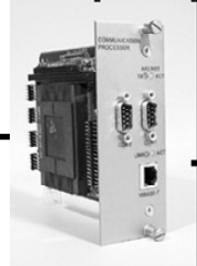
The Communication Processor requires two slots in a MOD HUB chassis.
