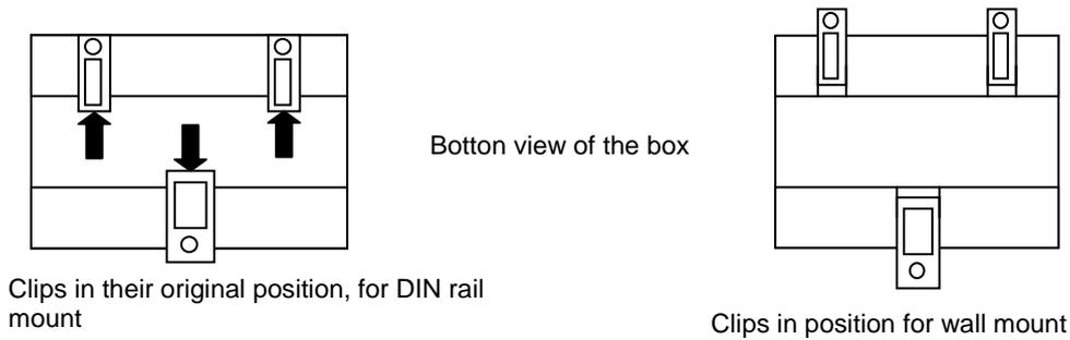
2. Use the holes of the clips to fix the box in the wall using screws. Use the template below for the wall holes.
