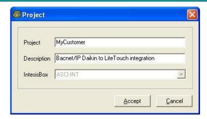
On *Accept*, a new folder will be created inside the projects folder with the name given to the project, this folder will contain the template configuration files if the project is a brand new one, or a copy of the configuration files if it is a copy of a selected one.
