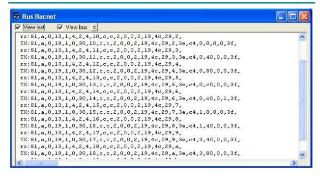
To monitor the communication between the gateway and the ASCII device, select the menu  $View \rightarrow Bus \rightarrow ASCI-INT$ . The ASCII communication viewer window will be opened. This window shows in real time all the communication frames between the gateway and the ASCII device as well as debugging messages referent to ASCII protocol sent by the gateway.
