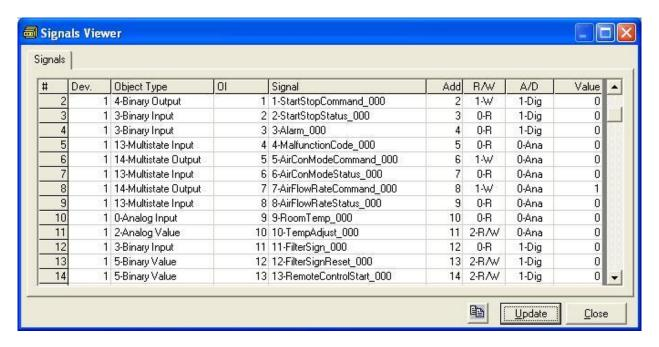
It is possible to force a specific value to any signal for test purposes, to do so just double click on the row and select the desired value and Accept in the Data Test window.
