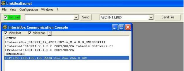
8. Open the ASCII Communication Viewer window (menu View -> Bus -> ASCII), force some point's polling from the ASCII device connected to IntesisBox, and check that there is communication activity, some TX frames and some other RX frames. This means that the communication with the ASCII device is ok. In case there is no communication activity between IntesisBox and the ASCII device check that ASCII device is operative and well connected to the IntesisBox.
