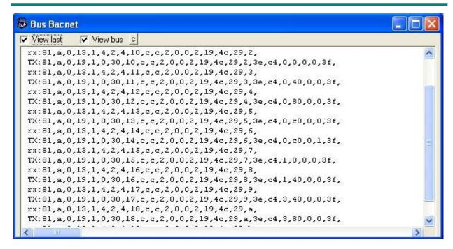
In case there is no response from the BACnet devices to the frames sent by IntesisBox check that they are operative and reachable from the network connection used by IntesisBox, check the IntesisBox's BACnet IP interface using any commercial BACnet browser connected to the same Ethernet network. See details for the communication cable between IntesisBox and BACnet system in section Connections of this document.
